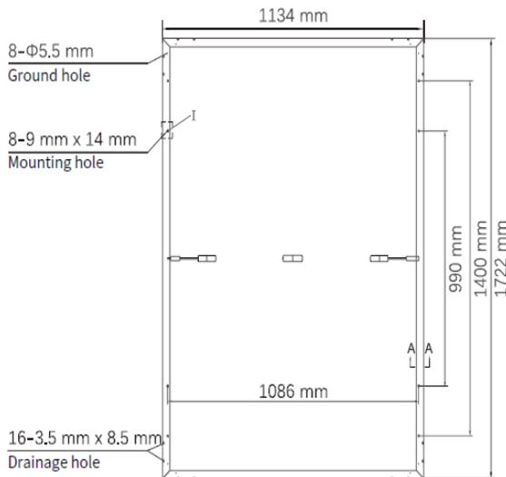
**Fig. 16** Grounding hole location on panel frame
